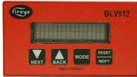
The NEXT key is used to scroll down through the various menus and is also used to increment the value when in the modify mode. The BACK key is used to scroll up through the menus and is also used to decrement the value when in the modify mode. The MODE key is used to enter a sub-menu when the displayed item indicates a sub-menu with a right facing arrow and also to exit the sub-menu and move on to the next main menu item. The RESET/MDFY
