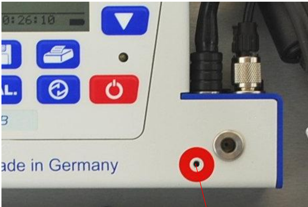
Fresh air opening
