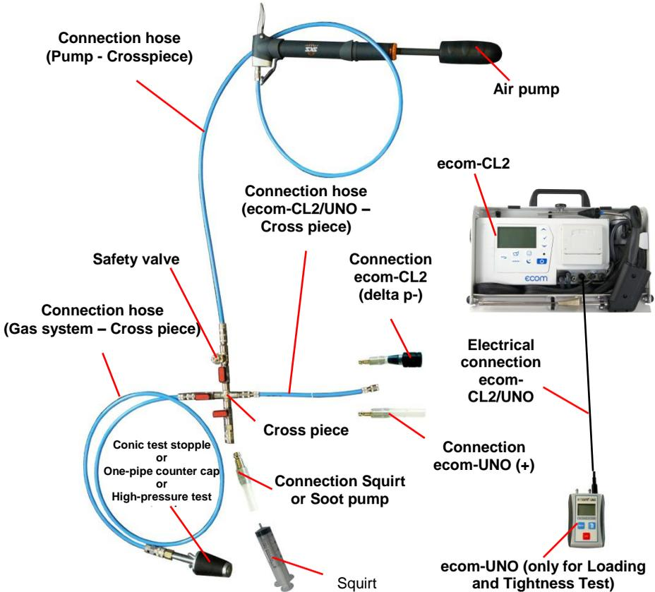
Call up the menu „**Pressure Tests**“ with the pre-programmed measurement routines „**Pressure Test**“, „**Loading Test**“, „**Tightness Test**“ and „**Usage property**“. Parameters to each measurement routine can be adjusted in the menu „**Setup**“.
