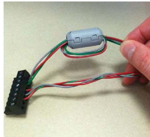
Fig. 3. Clamp filter in place.
